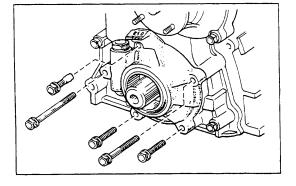
REMOVE OIL PUMP ASSEMBLY Remove the five bolts and the oil pump assembly.
